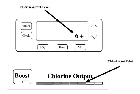
Your VX Salt chlorinator will always attempt to adjust the output so that the actual output level matches set point level. At times when the Chlorine output level is lower than the set point, check the salt level in your swimming pool at your local pool shop. Alternatively, you may have a low voltage supply to the chlorinator (less than 240Volts) or the water may be colder than usual.
