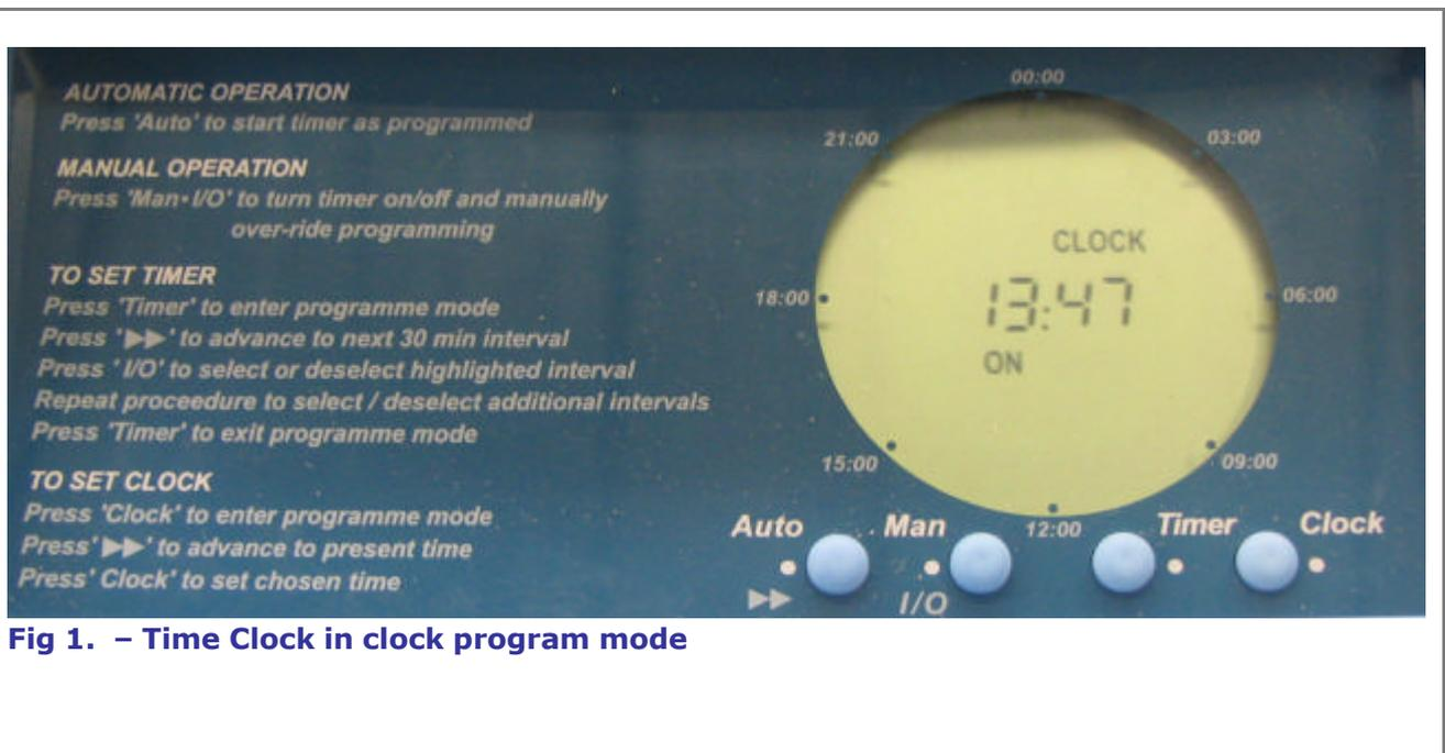
Fig 1. – Time Clock in clock program mode
